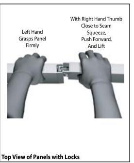
The first level of components contains panel locks that are located at the top of the panel for extra stability and a seamless connection. When disassembling panels, twist top connection slightly and lift right panel upward.
