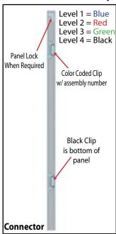
Each component has 2 clips, the lower clip is ALWAYS black. The top clip is color coded to distinguish the level. The color coded clip also contains the numbered label.
