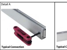
Most horizontal extrusion connections have a patented expandable lock. This lock inserts into the groove of an opposing extrusion. Tightening the lock with the Hex Key Tool expands the lock and creates a strong positive connection.
